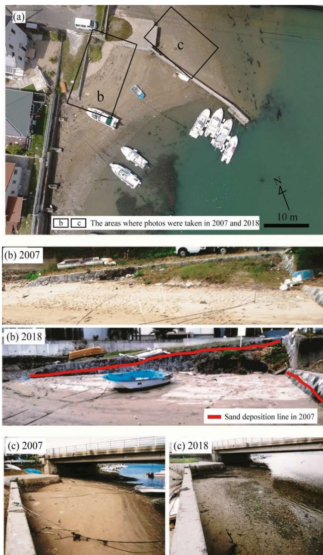
Figure 2.8 Comparison of beach morphology and condition at Site 2 between 2007 and 2018. (a) Birds-eye view, showing the two spawning areas, b and c. (b) Comparison of the sand accumulation at b area in 2007 (above) and in 2018 (below). (c) Comparison of the sand accumulation at c area in 2007 (left) and in 2018 (right).
