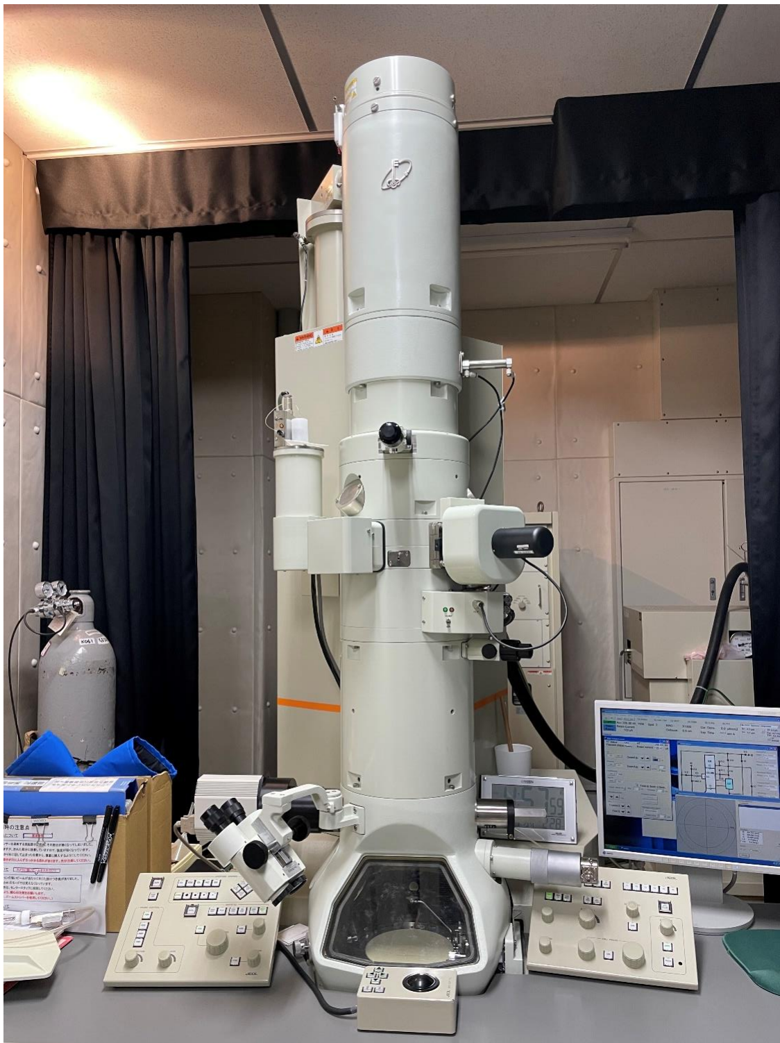
Figure 3-3. A conventional TEM (JEM-2100HC, JEOL Ltd.) in Kyushu University.
