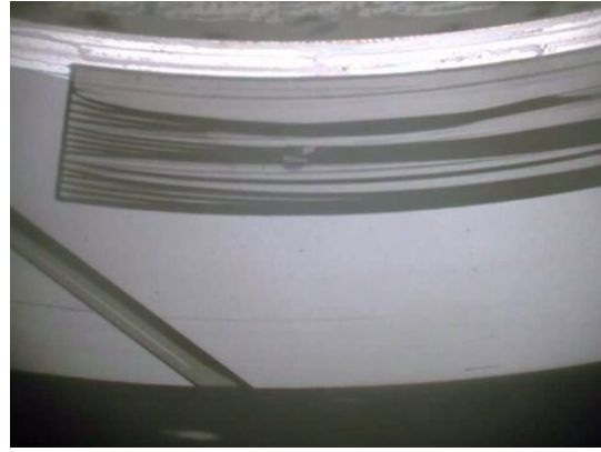
b) Time : 60sec, Cavitation pressure:90kPa(abs.)
