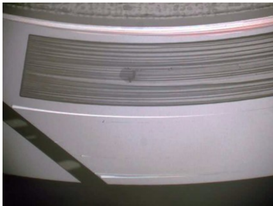
c) Time : 150sec, Cavitation pressure:27kPa(abs.)
