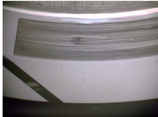
d) Time : 300sec, Cavitation pressure:34kPa(abs.)
