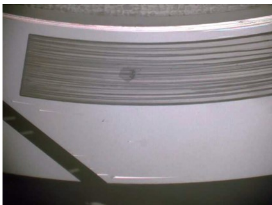
e) Time : 600sec, Cavitation pressure:28kPa(abs.)
