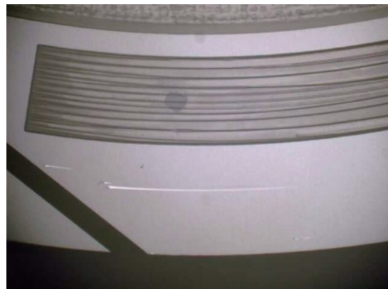
d) Time : 300sec, Cavitation pressure:60kPa(abs.)
