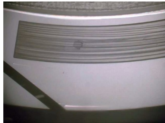
d) Time : 300sec, Cavitation pressure:27kPa(abs.)
