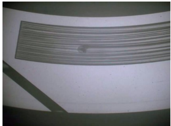
d) Time : 300sec, Cavitation pressure:25kPa(abs.)
