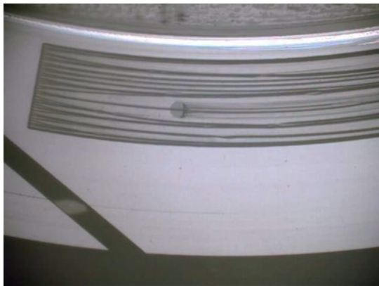
c) Time : 150sec, Cavitation pressure:49kPa(abs.)
