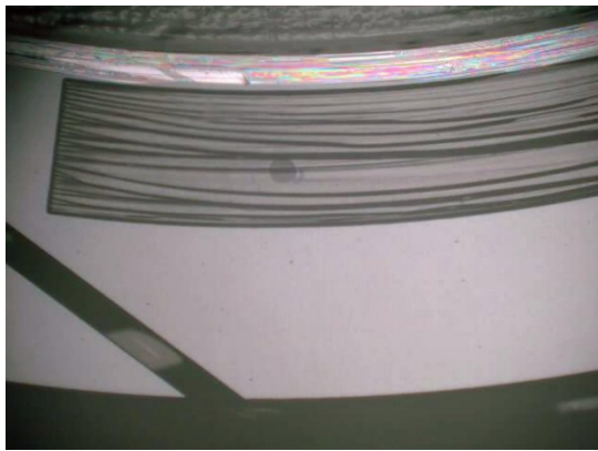
c) Time : 150sec, Cavitation pressure :75kPa(abs.)
