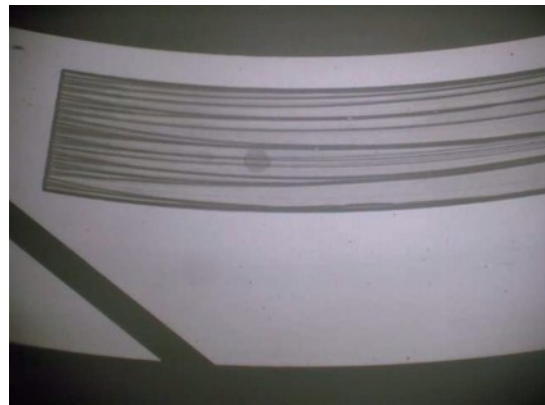
d) Time : 300sec, Cavitation pressure:68kPa(abs.)
