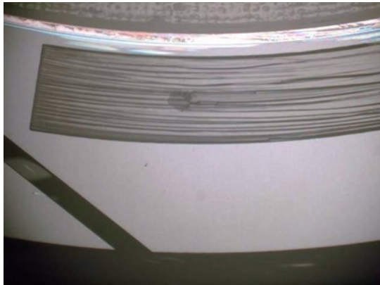
c) Time : 150sec, Cavitation pressure:34kPa(abs.)
