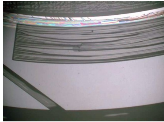
b) Time : 60sec, Cavitation pressure:86kPa(abs.)
