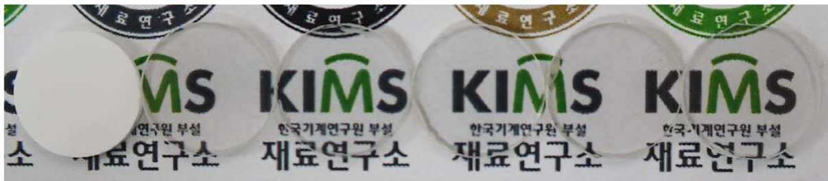
Fig. 4. Optical appearances of HIP treated \text{Y}_2\text{O}_3 ceramics hot-pressed at 1300, 1350, 1400, 1450, 1500, and 1550°C (2 mm in thickness) [26].
