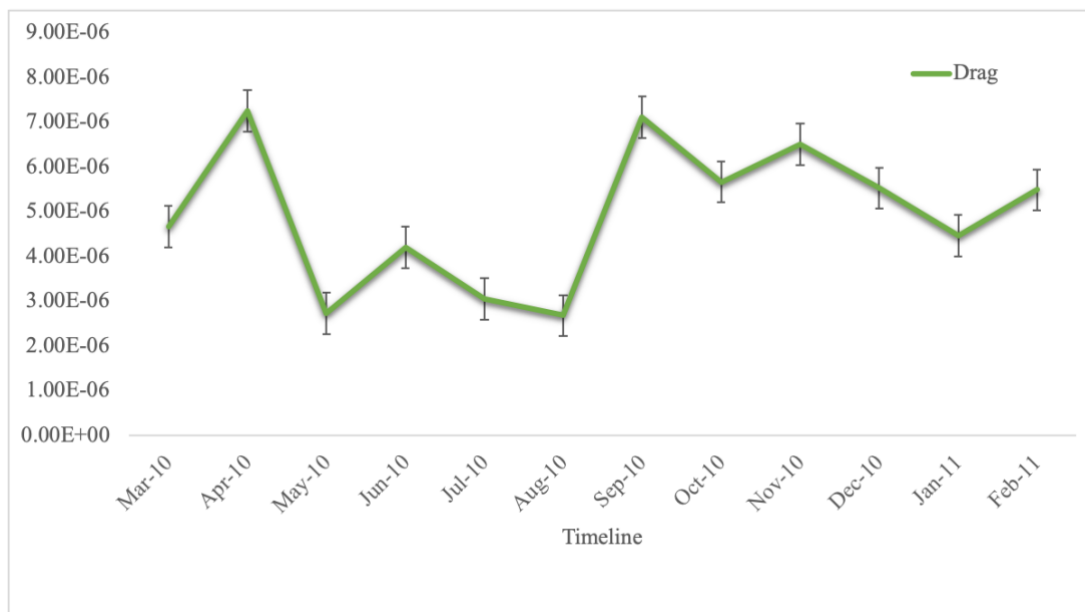
Figure 3.46 Atmospheric Drag on E-Sat for one year
