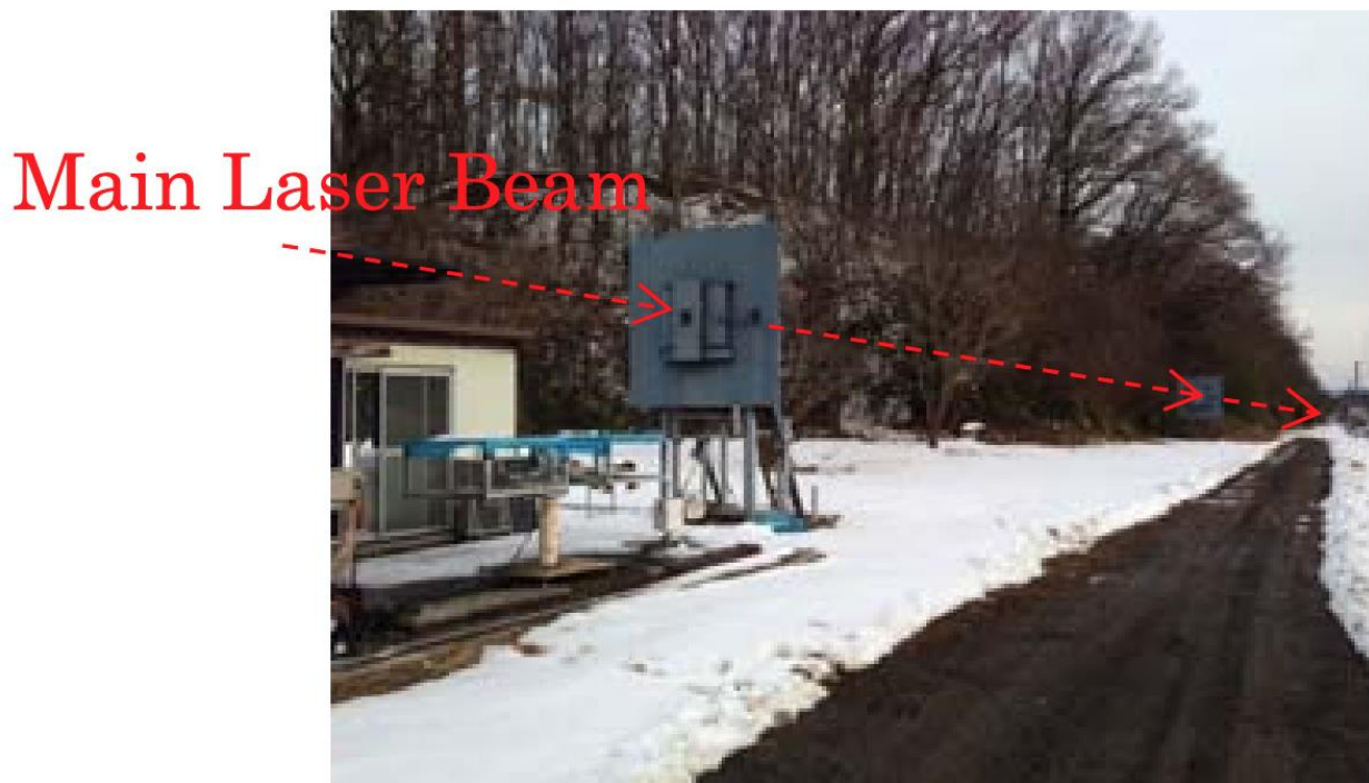
Figure 2.21 A 500 m horizontal laser transmission test at JAXA Kakuda Space Center
