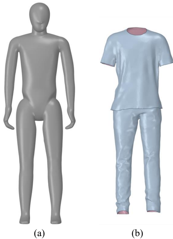
Figure 4-1. Three-dimensional (3D) digital model of thermal manikin and clothes: (a) Manikin and (b) T-shirt and Pants
