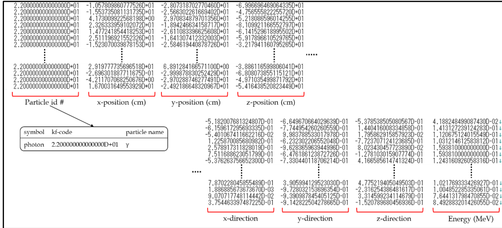
Fig. 5.3: Particle information dumped in a file. This information was recorded in the case of ^{47}\text{Sc} therapy and showing as an example from all other ‘dump’ files.
