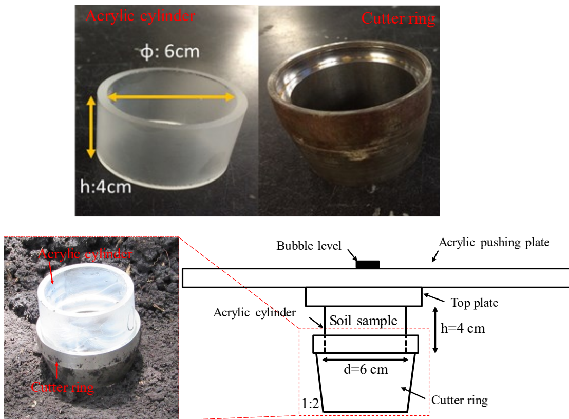
Fig 3.1 Sampling setup for undisturbed sample
