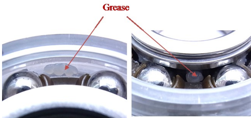
Fig. 3-3 The position of filled grease in a test bearing
