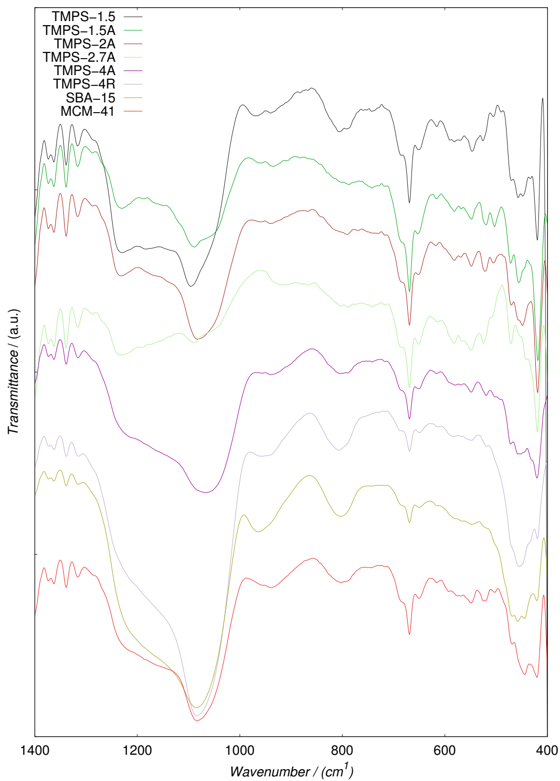
FIGURE A.4: FTIR analysis of the TMPS materials and regular mesoporous silica SBA-15 and MCM-41
