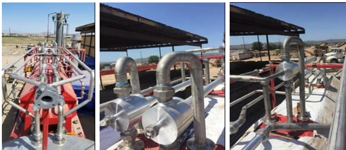
Figure 3. 8: Assembly of Ejector-Based System (GTI)
