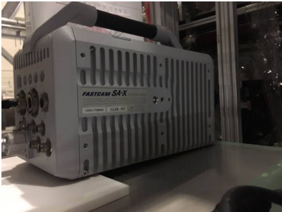
Figure 2.13 Photograph of fast camera. Model FASTCAM SA-X from PHOTRON, INC.
