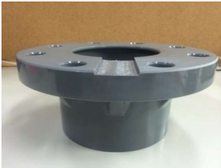
Figure IV-3 Slit on the flange for outflow of jet
