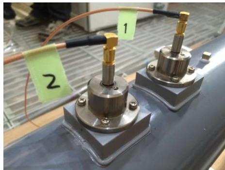
Figure IV-5 Installation of microphones
