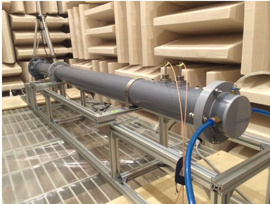
Figure IV-1 Acoustic impedance tube
