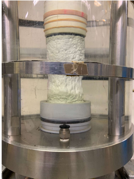
Photo 5.7 The necking appeared when Kuroboku pre-sheared to DA = 25.68\%
