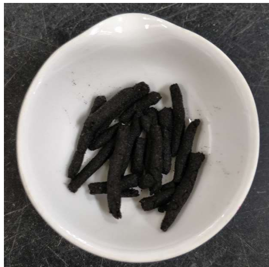
(b) Sample's preparation for Plastic Limit test
