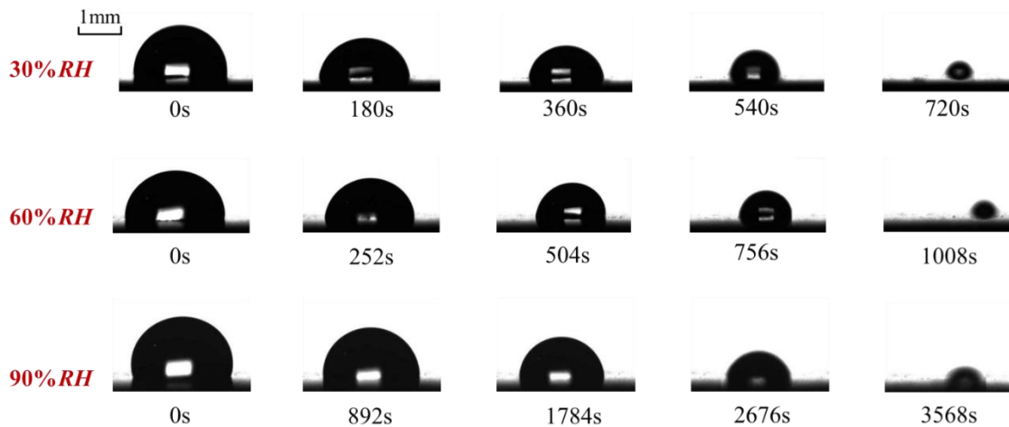
Figure 5.3 Profile evolution of pure water droplets during evaporation for ambient condition of 45°C and 30% RH , 60% RH , 90% RH , for \tau = 0, 0.25, 0.5, 0.75 and 1.
