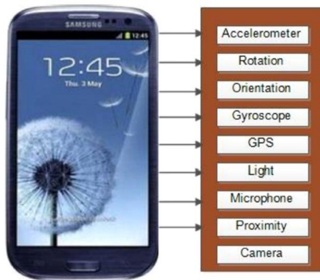
Figure 3: Smart Phone Sensors: Galaxy S4 and embedded sensors. [20]
