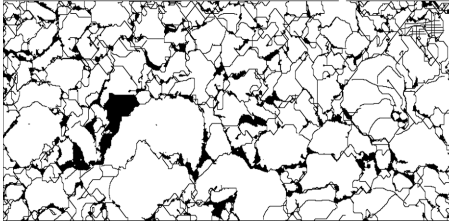
Fig. 5.2 The photograph after image analysis by Split-Desktop
