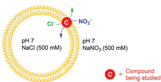
Figure 4-7. Schematic diagram of ISE \text{Cl}^- – \text{NO}_3^- exchange assay.
