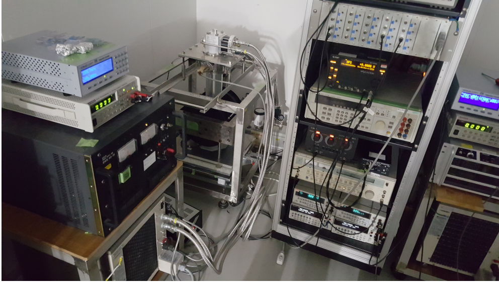
Figure 3.5: Lock-in measurement setup
