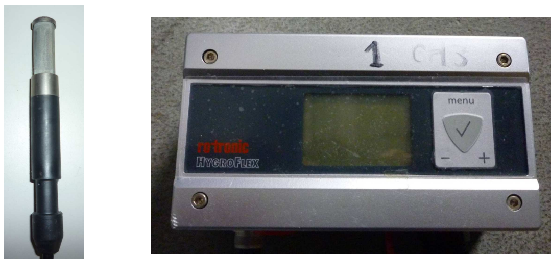
Fig.2.16 Picture of the humidity sensor and the converter.
