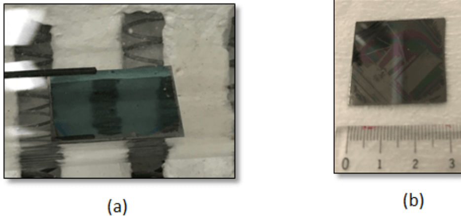
Fig. 3.7: \text{SiO}_2 sol-gel on Si substrate sample at (a) maximum annealing temperature (position 1 in Fig 3.5) showing no cracks while (b) sample with 8^\circ\text{C}/\text{min} cool down ramp (position 2 in Fig. 3.5) showing cracks across the whole sample
