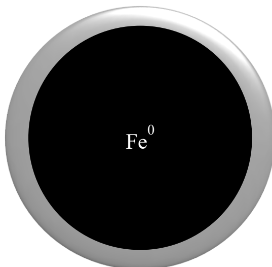
Figure 1.5 Core shell structure on nZVI
