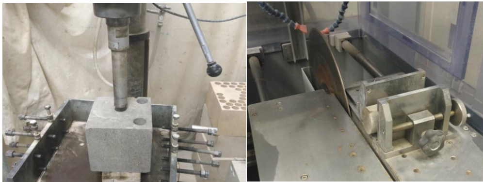
Figure 2-2. Coring bit (Left) and surface grinder (Right).
