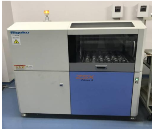
Figure 2-4. X-ray fluorescence equipment for rock composition measurement.
