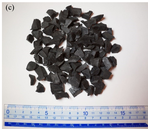
Figure 2.4 Tire chips samples: (a) TCH1 (b) TCH2 (c) TCH3
