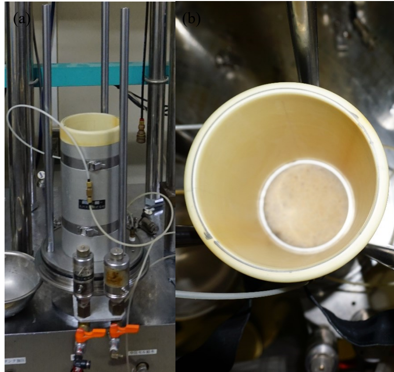
Figure 3.2 Split mold and rubber membrane: (a) Front view (b) upper view
