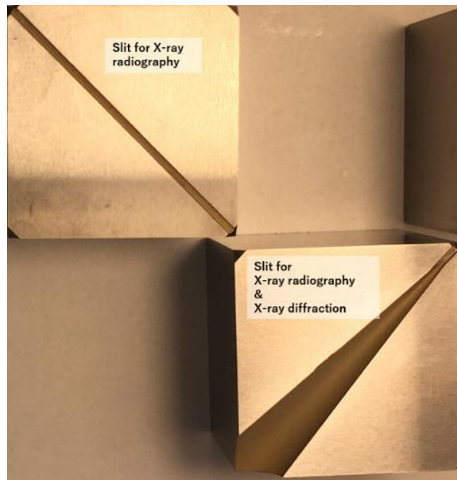
Fig. 1.18 Two types of slotted anvils used for the D-111 apparatus. The rectangular slotted anvils (upper left) and the rectangular and conically slotted anvils (lower right) are used at the upstream and downstream sides of the sample assembly, respectively.
