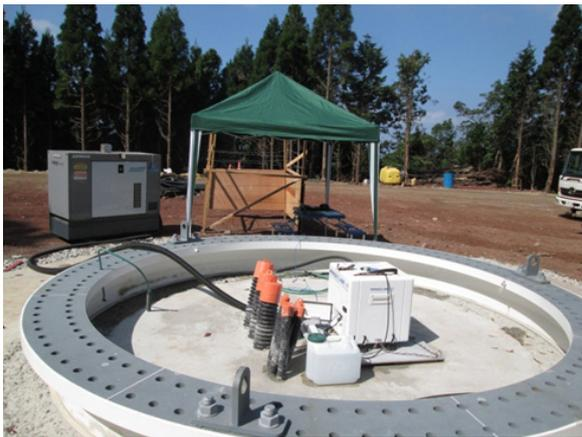
Fig.3 Wind resource measurement using LIDAR system
