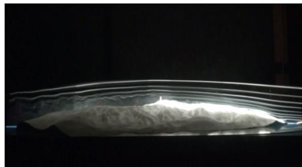
Fig.1 Wind tunnel test using actual topography model
