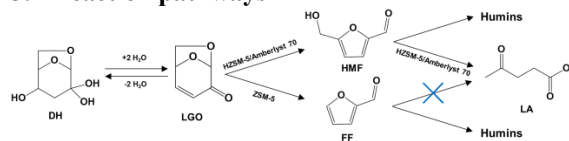
Scheme 1 LGO degradation in aqueous phase over solid acid catalysts.
