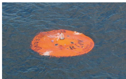
Fig. 2 Disk type underwater glider "BOOMERANG"
