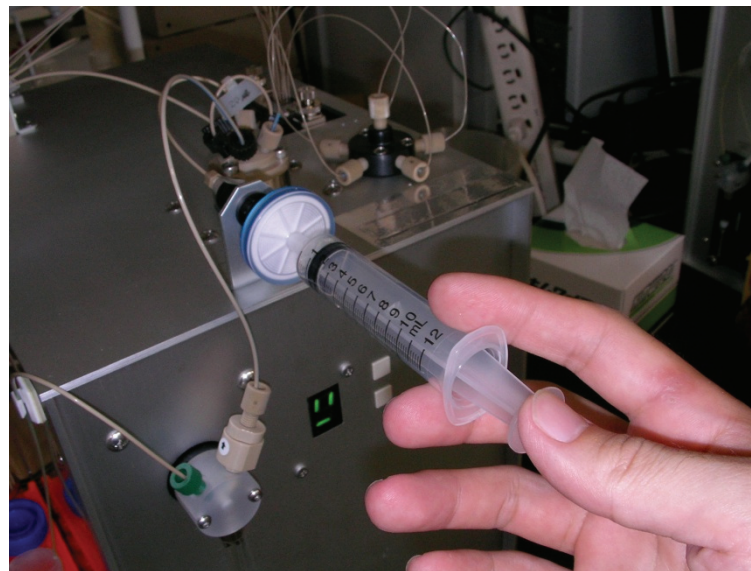
Injection into SPR sensor system (5 s)
