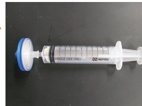
Extraction of explosives from wiper in syringe (30 s)
