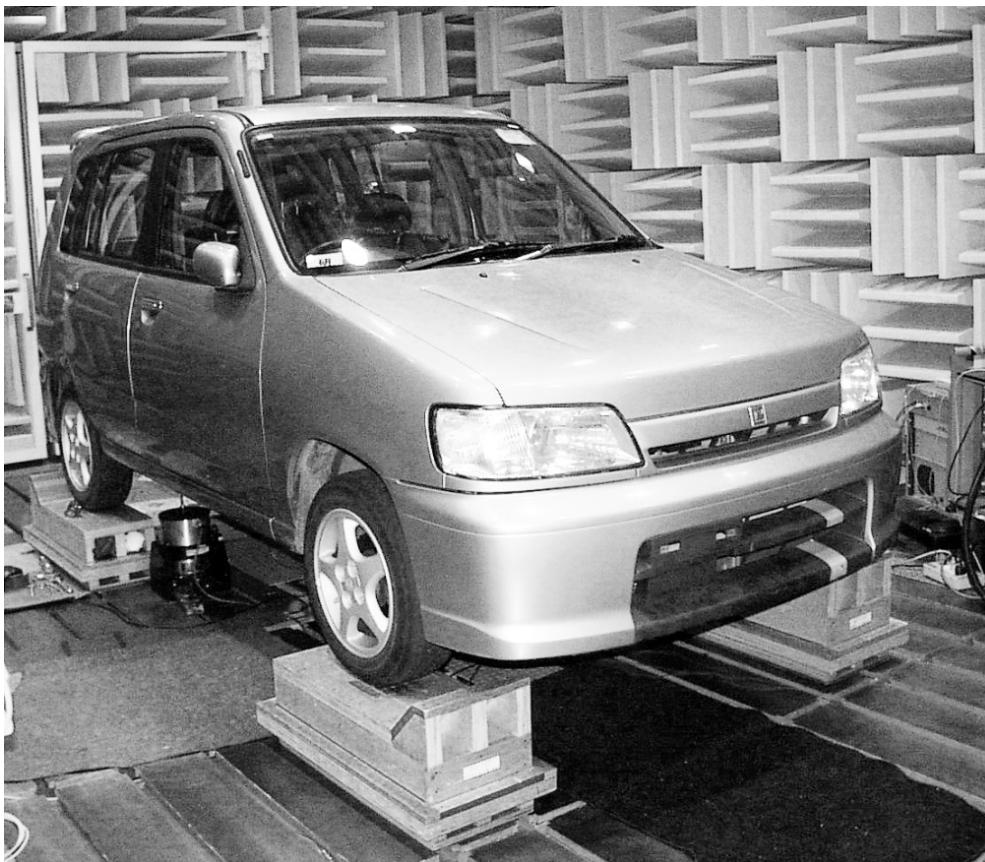
Fig. 3.1 The experimental vehicle in the semi-anechoic room.
