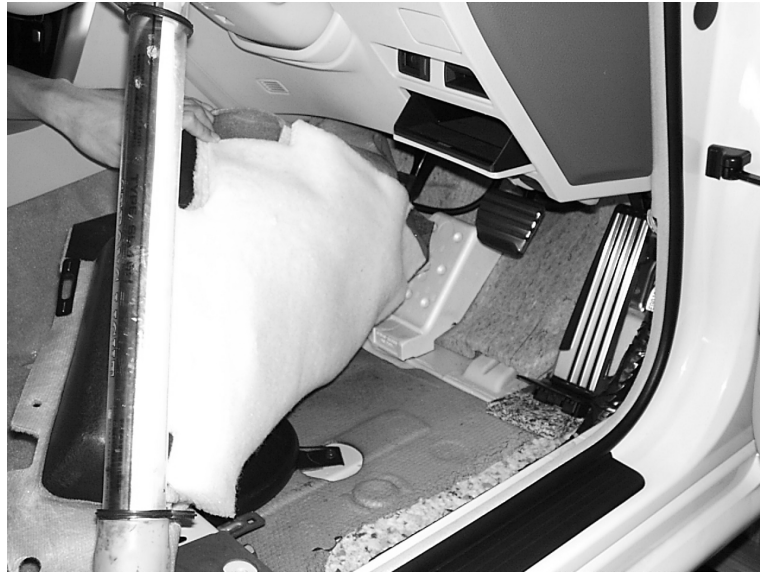
Fig. 1.2 Melting sheet under floor carpet. Melting sheet is attached in gray area.
