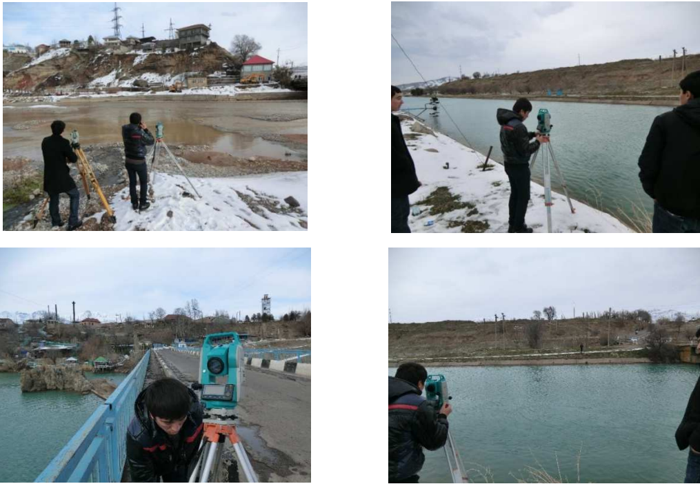
Figure 4.17 Measuring process of river cross section of Chirchik River
