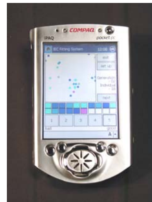
Figure 11: Graphical user interface of a PDA version of an IEC-based hearing aid fitting.
