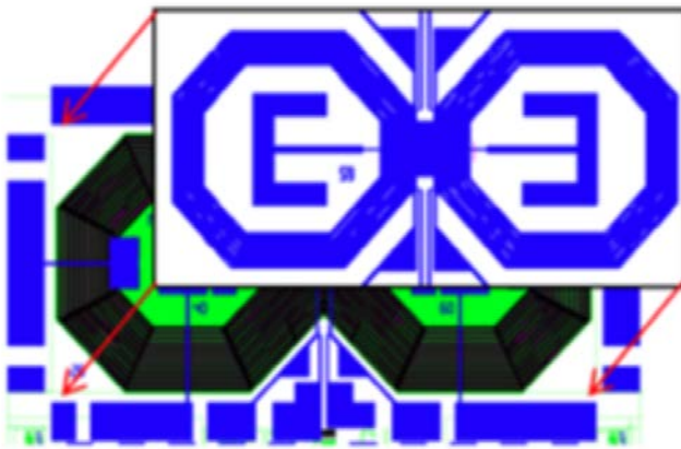
100 turn input coil (Flip-chip coupling)
