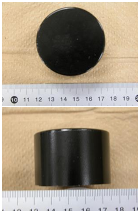
Fig.II-1-1 P0798 type simulated high-level waste glass.
