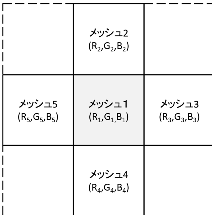
Fig. A.3 CC (Color Complexity) calculate area. Gray mesh indicates target mesh. CC was calculated as the standard deviation among target mesh and neighboring 4 meshes.
