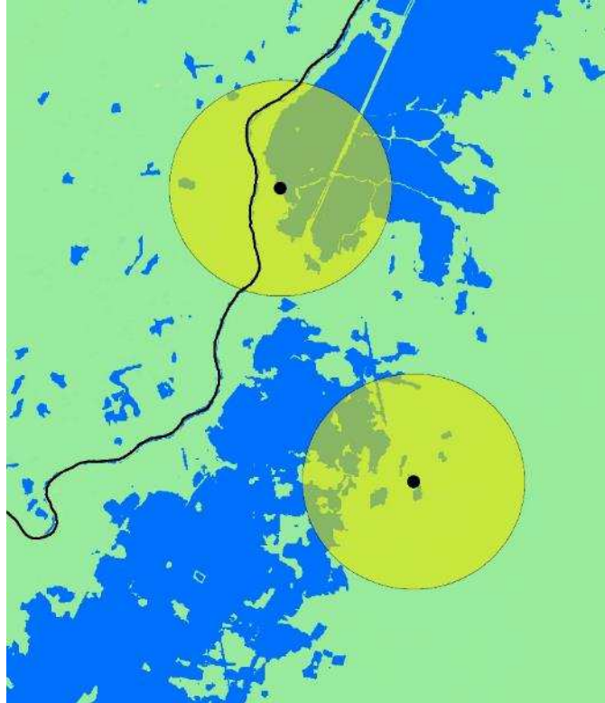
Fig. 2.3 The buffer shapes which extracted the flood plain area within. The blue areas are floodplains.
