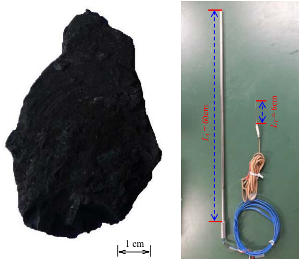
Figure 2- 13 Test coal size and thermocouple length definition
