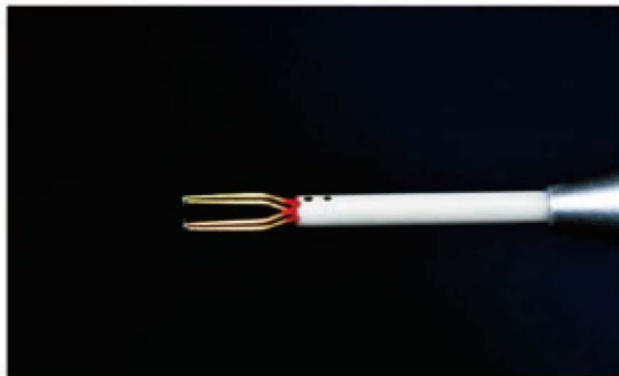
Fig. 6 Split-fiber probe, capable of detecting reversed flow
