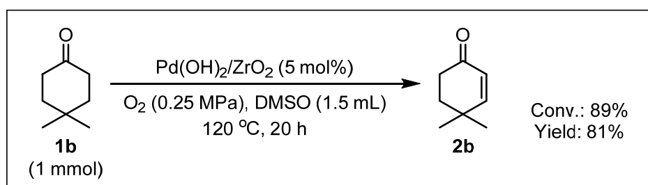
Scheme 3.4 Synthesis of 4,4-dimethylcyclohexenone from 4,4-dimethylcyclohexanone over Pd(OH) 2 /ZrO 2 .
