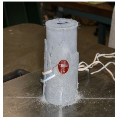
Figure 5.4 Compressive failure of ECC
