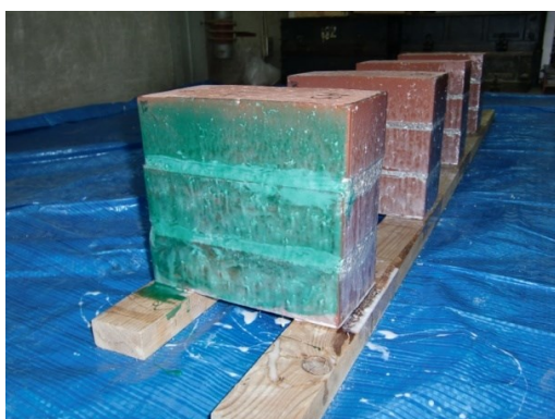
Figure 5.41 Application of adhesive
