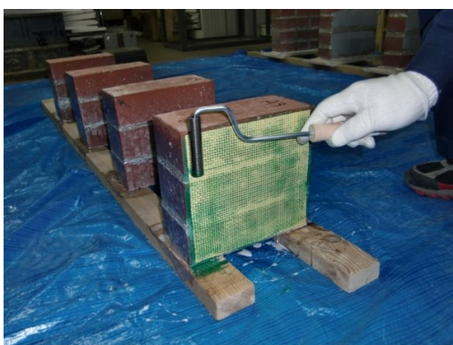
Figure 5.42 Removing air with roller
