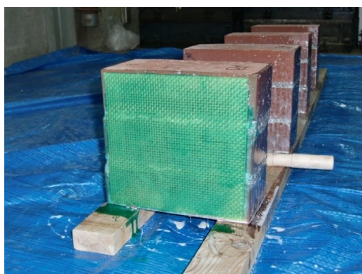
Figure 5.43 Coating with adhesive
