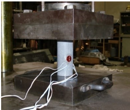
Figure 5.3 Compressive test on ECC
