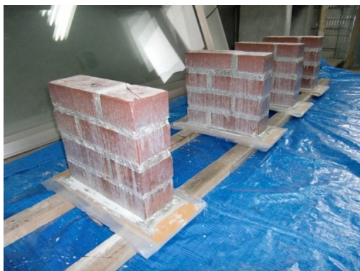
Figure 5.39 Application of primer
