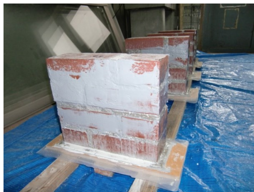
Figure 5.40 Surface treatment using putty
