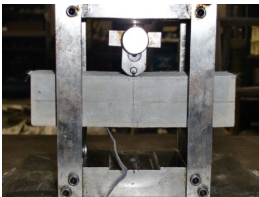
Figure 5.5 Bending test on ECC
