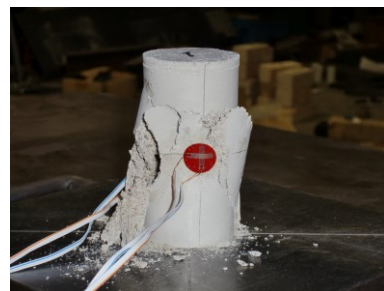
Figure 5.12 Compressive test on bed joint mortar
