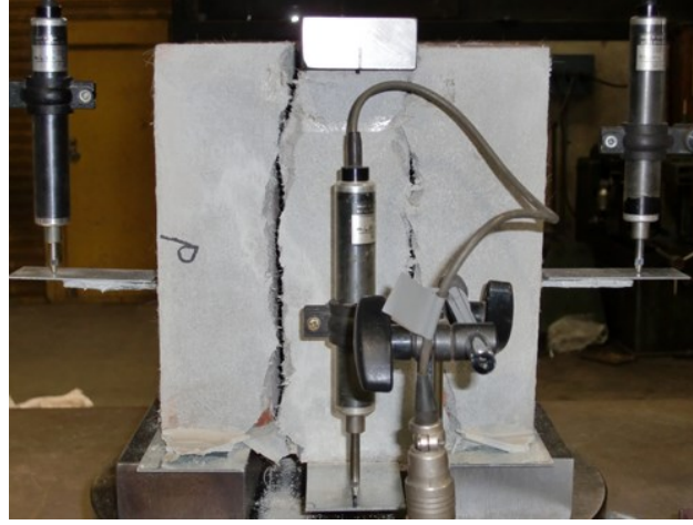
Figure 6.1 Crack propagation in ECC retrofitted triplet specimens
